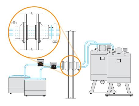
The AdvantaPass system is customizable to fit various wall thicknesses and can be adapted for floor-to-ceiling conveyance. It manages multiple tubing apertures and purge ports through a single wall portal.
