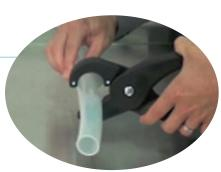
Specific cutting techniques are strongly recommended for APHP. The tubing must be cut with a chevron style cutter at a 90 degree angle to the tubing. View cutter product details at https://www.lislecorp.com/ specialty-tools/hose/hose-cutter.
